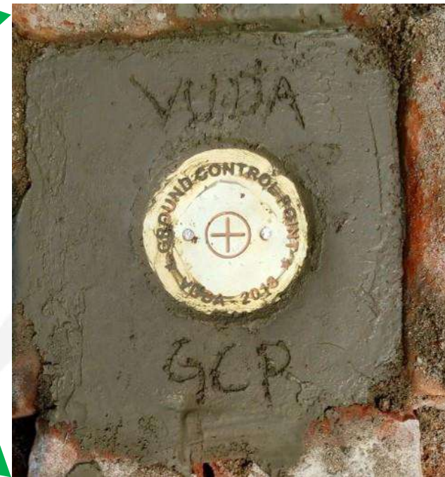
Control Point Plate on Ground
